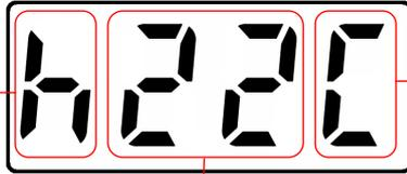
Temperature can be displayed in °C or °F. This can be changed by SW1.
